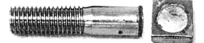
The manner in which a bolt or screw breaks during testing is as important as to whether or not it meets or exceeds its minimum strength requirements. Even if a bolt breaks at twice its minimum strength requirement, but the break is where the head connects to the shank the bolt is unacceptable.
